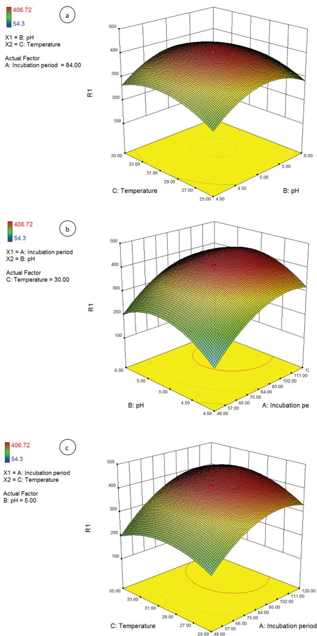
**Figure 4.** (a). Response surface plot of temperature vs. pH on ethanol production (time was kept constant at 72 h). (b). Response surface plot of pH vs. incubation period on ethanol production. (c). Response surface plot of temperature vs. incubation period on ethanol production.
