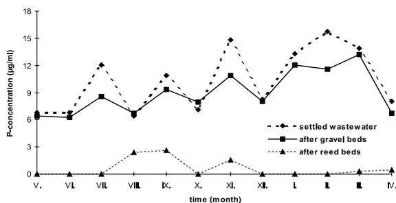
Figure 1. P concentrations of the water samples ( $\mu\text{g/ml}$ ).
