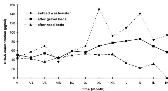
Figure 2.  $\text{NH}_4\text{-N}$  concentrations of the water samples ( $\mu\text{g/ml}$ ).
